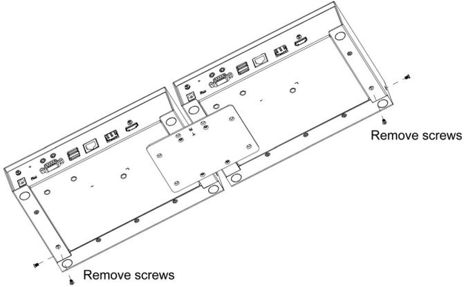
3. Use the screws in step 2 to install the left and right mounting brackets.
