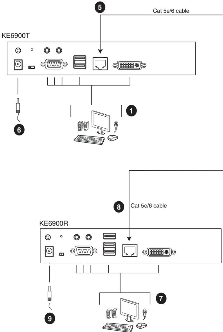
**Note:** The diagram above shows the KE6900T and KE6900R. The KE6940 installation is the same except that an additional DVI monitor can be connected at each end for a dual-view display setup.
