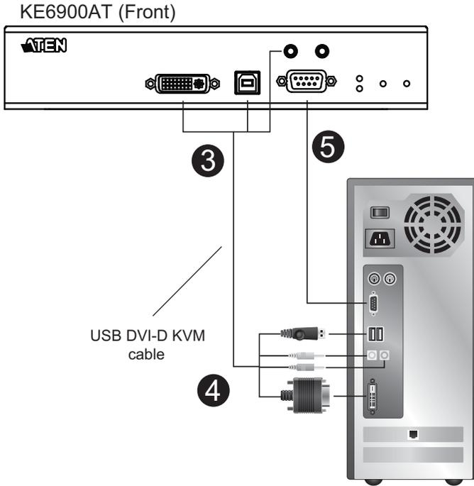
**Note:** The serial port on the Transmitter (shown above) connects to the computer; the serial port on the Receiver (not shown) connects to a serial device (optional).
