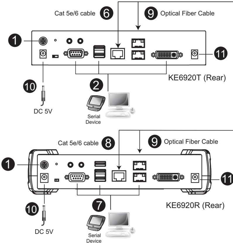
**KE6920 / KE6922 Point-to-Point Installation 2 of 2**
