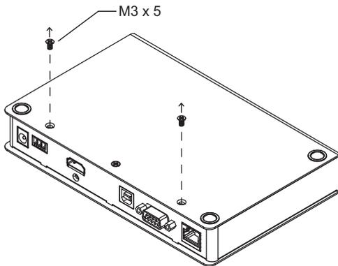
2. Use the screws from step 1 to screw the mounting bracket to the bottom of the Transmitter as shown below:
