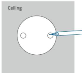
2. Drill holes with a  $5/16"$  (8 mm) drill bit.
