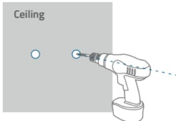
3. Align the holes on the mounting plate with those in the ceiling. Insert the anchors into the holes; anchors are necessary for walls that are made out of hard materials such as concrete, brick, or stucco. Fix the screws with a Phillips-head screwdriver to fasten the mounting plate to the ceiling.
