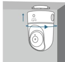
To mount the eufy Indoor Cam on a wall, we recommend using the mounting bracket (not provided) as the illustration below.
