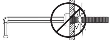
ENG Do not overtighten screws.
