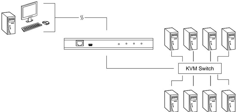
The CN8000A expands on previous models by providing a dedicated RS-232 port for modem access or serial console management, a PON port to attach a Power Over the NET™ device and a Laptop USB Console port for easy console access from a laptop.
