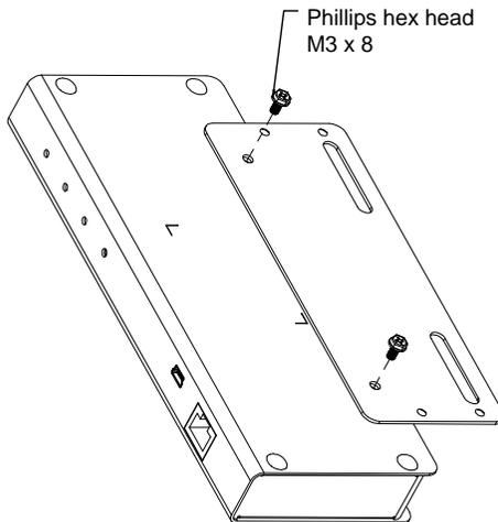
3. Screw the bracket into any convenient location on the rack.
