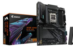
**Product name :** X870E AORUS ELITE X3D Motherboard - Supports AMD Ryzen 9000 CPUs, 16+2+2 Phases Digital VRM, up to 9000Hz DDR5 (OC), 2xPCIe 5.0 + 2xPCIe 4.0, Wi-Fi 7, 5GbE LAN, USB 4
