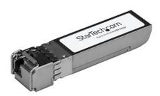
The SFP-10GB-BX-D-STA-ST is a MSA compliant downstream fiber SFP+ transceiver which pairs with StarTech.com's SFP-10GB-BX-U-STA-ST. They are designed, programmed and tested to work with 10GBASE-BX compatible MSA switches and routers. The SFP+ transceiver module supports a maximum distance of up to 10 km (6.2 mi) and delivers dependable 10 GbE connectivity over fiber cabling.
