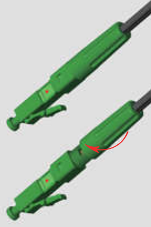
10. Screw tight the tail boot, complete the assembly.
