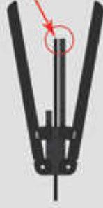
2. Insert the cable into the cable stripper, strip the cable as per the markings.
