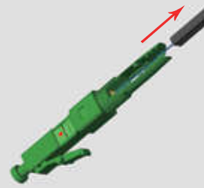
( 3 ) Draw out the fiber, complete the repeat assembly.
