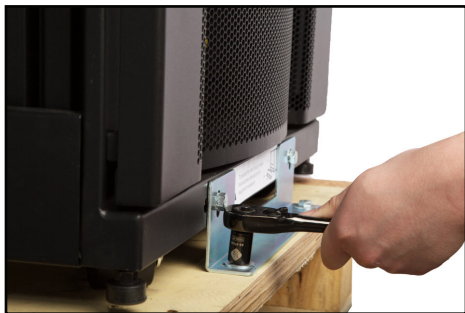
Removing the Bolts
