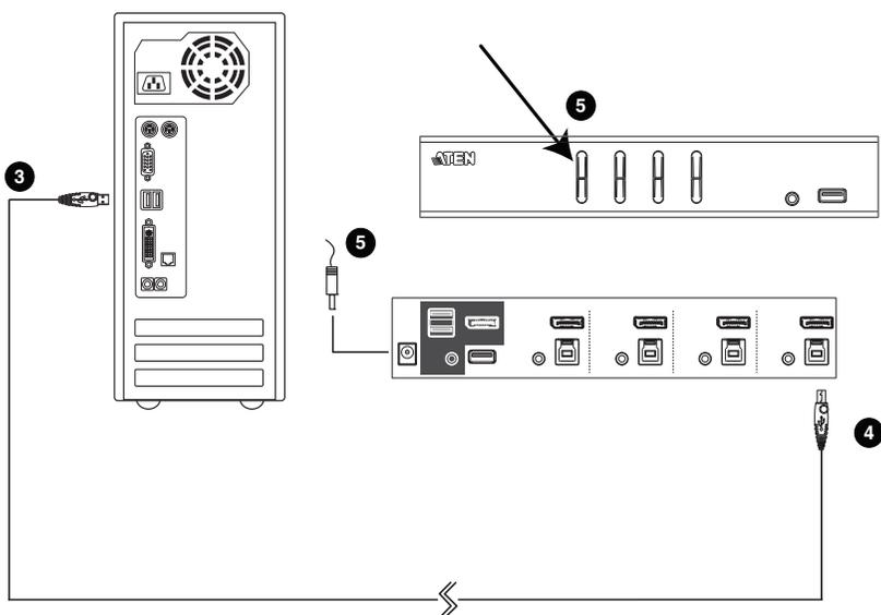
4. At the other end of the USB cable, connect the USB Type B connector to the Type B USB port in the Port 1 KVM section.
