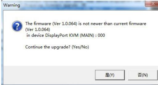
If you did not enable *Check Firmware Version*, the Utility installs the upgrade files without checking whether they are a higher level, or not.
