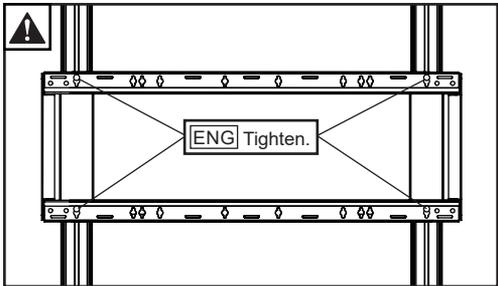
**ENG** Cross supports must center on vertical leg supports.
