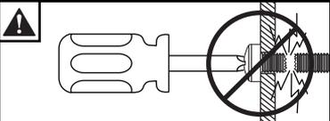
ENG Do not overtighten screws.
