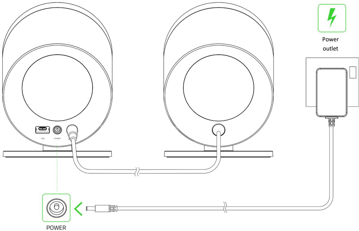
3. Connect the regional power cord to the power port on the subwoofer and plug it into a power outlet.
