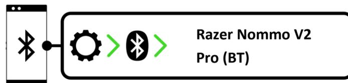
3. Wait until both devices are connected. The status indicator will turn solid blue to indicate that the gaming speakers are now connected to your device. In Bluetooth mode, the rear projection lighting will only light up according to your mobile device's current audio level (Audio reactive).
