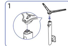
Put the stand base onto the stand neck as the direction shown in the figure. Check that the stand neck is firmly connected.
