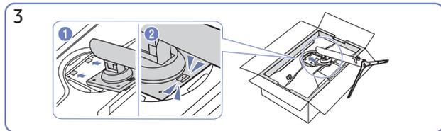
Push the assembled stand into the main body in the direction of the arrow as shown in the figure.
