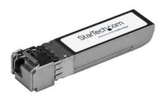
The SFP-10GB-BX-U-STA-ST is a MSA compliant upstream fiber SFP+ transceiver which pairs with StarTech.com's SFP-10GB-BX-D-STA-ST. They are designed, programmed and tested to work with 10GBASE-BX compatible MSA switches and routers. The SFP+ transceiver module supports a maximum distance of up to 10 km (6.2 mi) and delivers dependable 10 GbE connectivity over fiber cabling.
