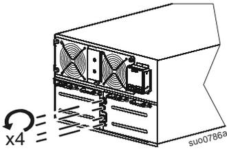
**2** Disconnect and remove four battery modules.
