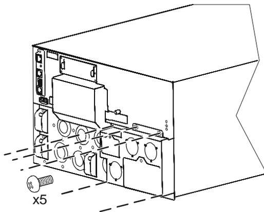
Install strain reliefs (not supplied), for the hardwire configuration that will be used.
