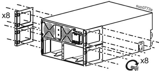
**2** Install the rails. Follow the rail installation instruction in the rail kit. Install six cage nuts.
