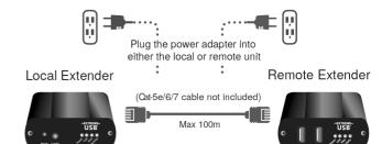
Note: Flexible power is different from Power over Ethernet (PoE). Ensure that the Cat-5e/6/7 cable is only connected between the Local and Remote Extenders.
