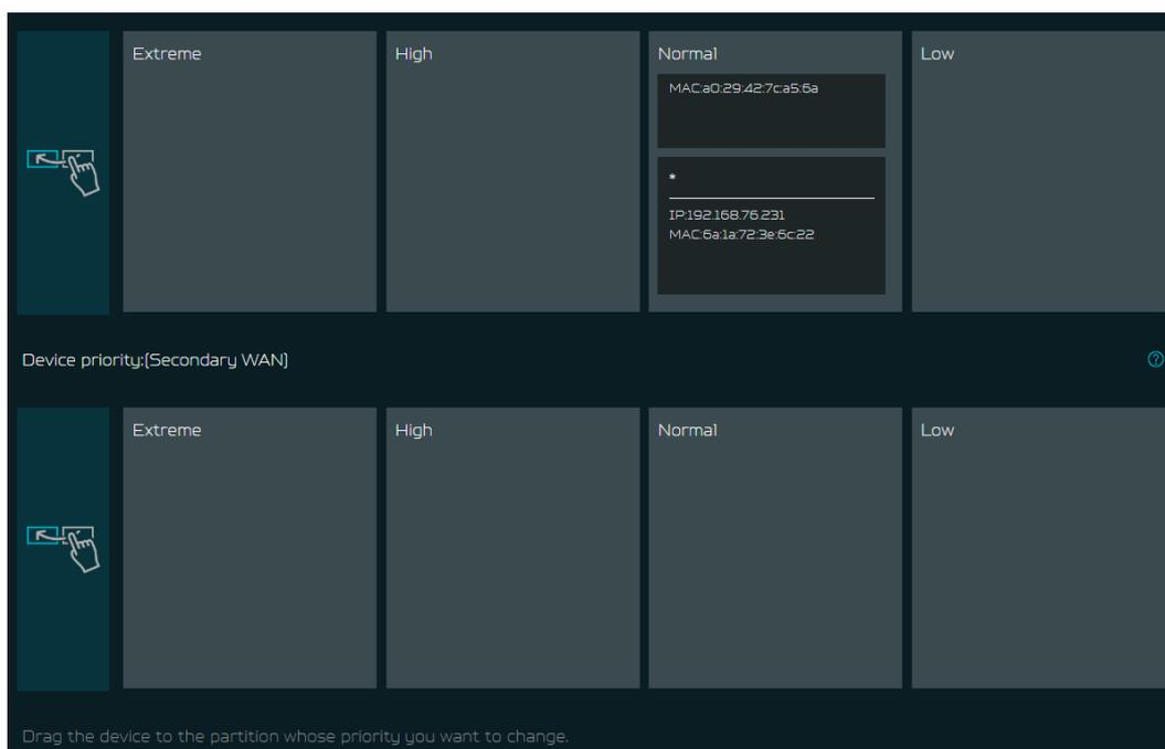
For the upload and download **bandwidth** configuration, please contact your ISP to get the exact value of the upload and download bandwidth. Once the bandwidth is configured, QoS will reserve the bandwidth according to the weighting percentage of each priority queue.
