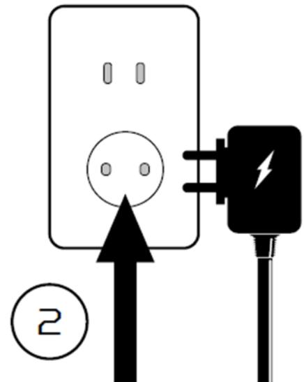
2.3. Plug in the Internet cable and power ON the device
