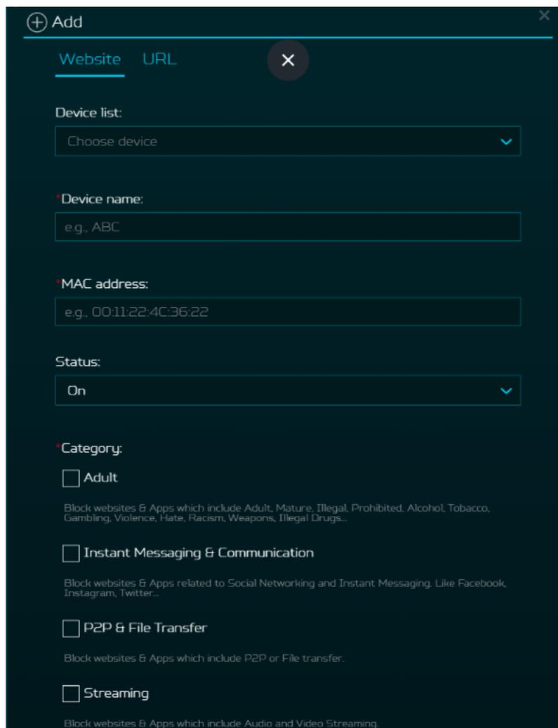
Under the URL tab, you can enter the device list, device name, its MAC address and URL, which you want to forbid access to e.g. www.aaaa.com. Or you can add a keyword e.g. AAAA to forbid any URL containing the keyword.
