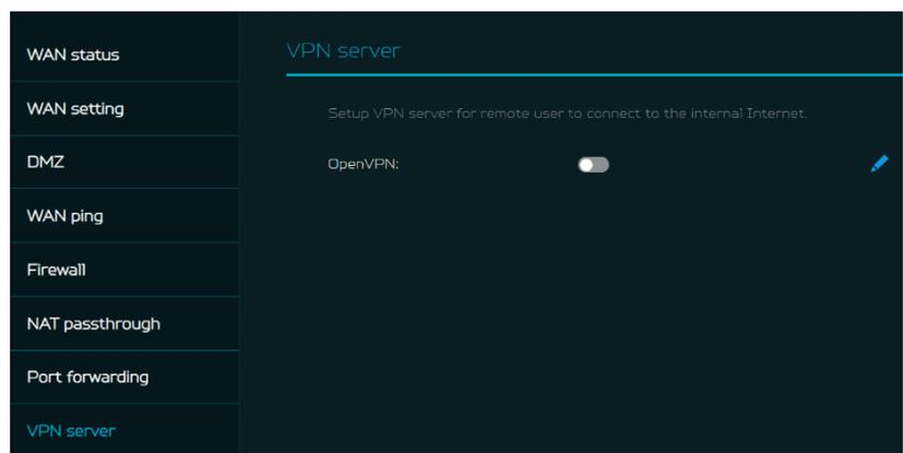
**Open VPN** is SSL VPN and uses a chosen UDP or TCP port, allowing for flexible configuration choices. User access consists of two different options; Home network, Internet and home network. Users can also export OpenVPN configuration file (client.ovpn).
