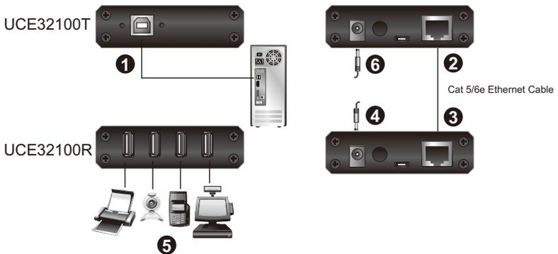
1. Connect the UCE32100T's USB Type-B Port to a USB port on the computer using a USB 2.0 cable.
