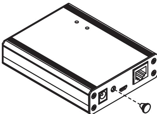
2. Insert the DC Jack Lock component A into the hole as pictured below.
