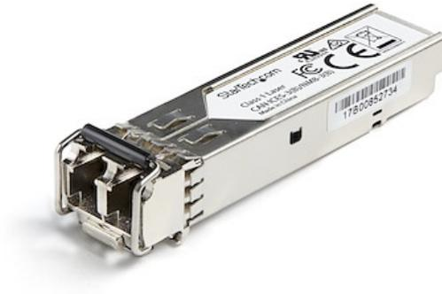
The CTPSFP1GELXS is a Juniper CTP-SFP-1GE-LX compatible fiber transceiver module that has been designed, programmed and tested to work with Juniper brand switches and routers. It delivers dependable 1 GbE connectivity over fiber cable, for 1000BASE-LX compliant networks, with a maximum distance of up to 10 km (6.2 mi).
