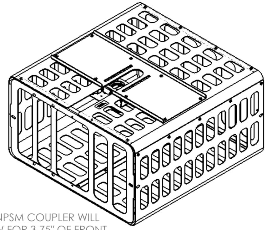
1.5" NPSM COUPLER WILL ALLOW FOR 3.75" OF FRONT TO BACK ADJUSTABLE SHIFT
