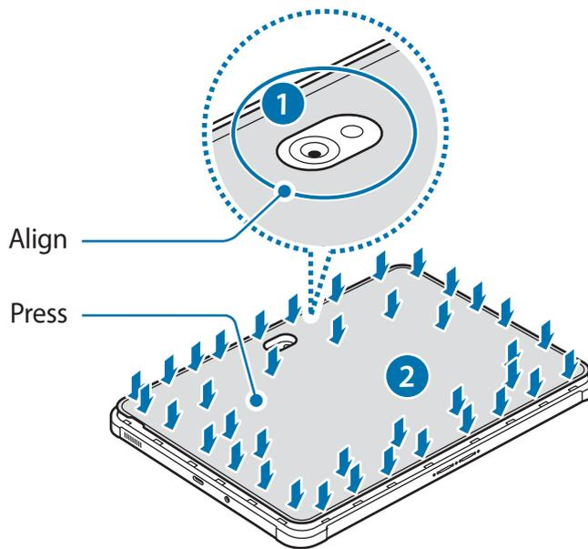
**!** Ensure that the back cover is closed tightly to prevent water and dust from entering the device. Open or loose back cover may allow water and dust to enter the device and cause damage.
