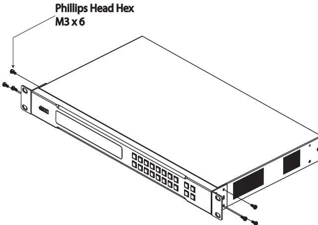
2. Position the unit in the front of the rack and align the holes in the mounting brackets with the holes in the rack.
