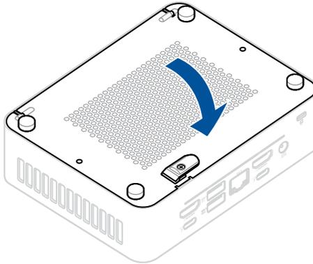
2. Secure the bottom cover by tightening the latch lock screw.
