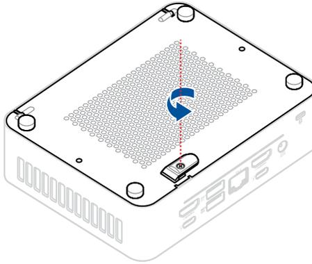
2. Lift the latch lock to unlock the bottom cover.
