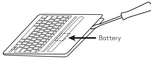
2. Detach battery from circuit board and remove battery.
