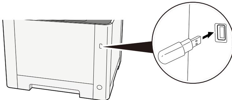
When the machine recognizes the USB drive, the message "USB Drive is recognized. Displaying files." appears.
