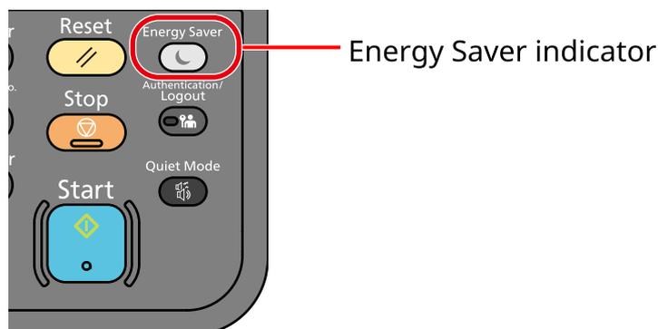
If print data is received during Sleep, the machine automatically wakes up and starts printing.
