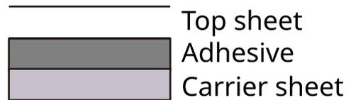
Labels consist of three layers as shown in the illustration. The adhesive layer contains materials that are easily affected by the force applied in the machine. The carrier sheet bears the top sheet until the label is used. This composition of labels may cause more problems.
