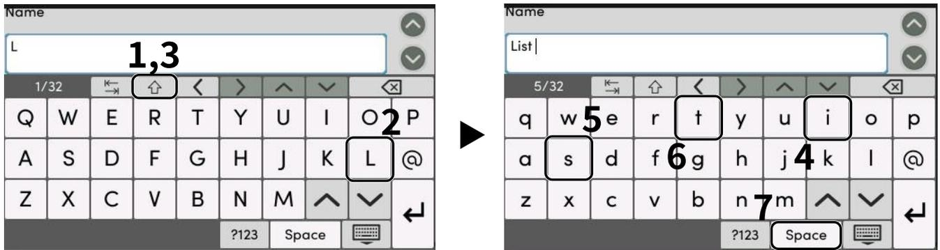
To switch between upper case and lower-case, select the Shift key.
