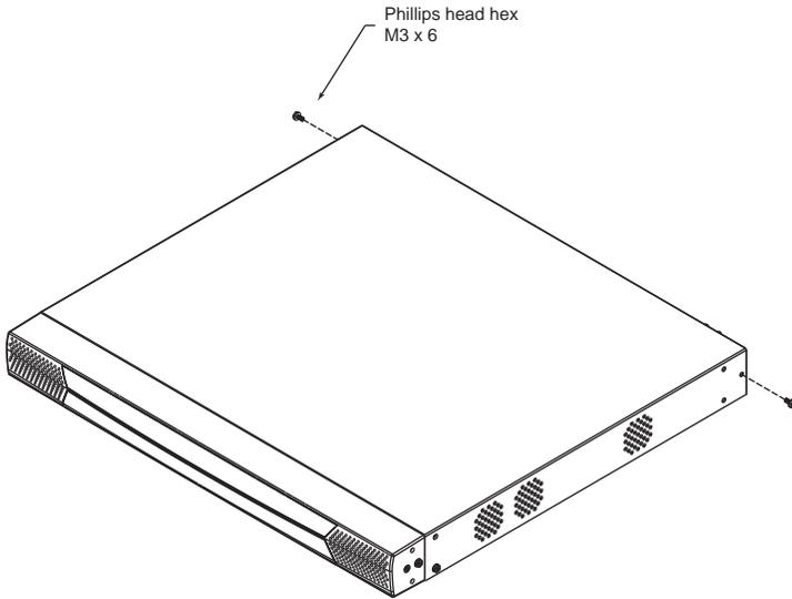
2. Use the M3 x 8 Phillips head hex screws supplied with the rack mounting kit to screw the rack mounting brackets into the rear of the unit.
