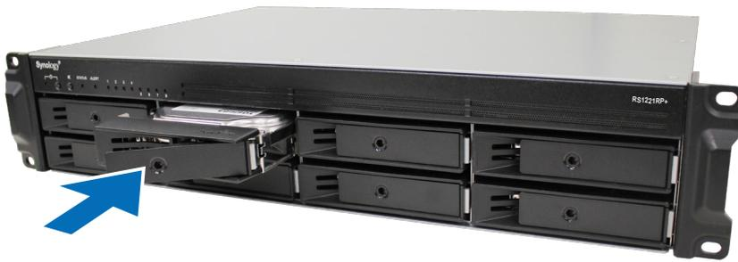
**Note:** Make sure that the drive tray is completely inserted. Otherwise, the drive might not function properly.
