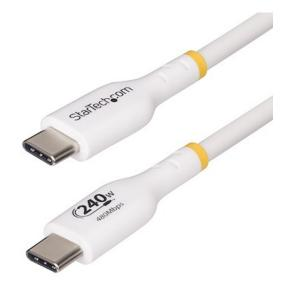
Connect a charger to a USB Power Delivery (PD) 3.1-enabled device, using this USB-C Charging Cable. The USB-C charger cord delivers up to 240W of Extended Power Range (EPR) Power Delivery and 5A output for fast charging. The connector markings enable quick visual identification, distinguishing this cable from other similar-looking or unmarked USB-C cables. Eliminate guesswork and always choose the appropriate Type-C cable to support full 240W charging.
