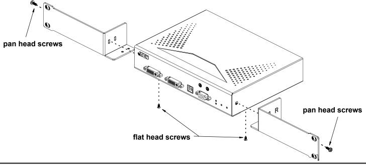
4. Screw the mounting brackets to the rack. The example used in the diagram below is a KE Sereis transmitter unit, the procedure for connecting to a receiver unit is identical.
