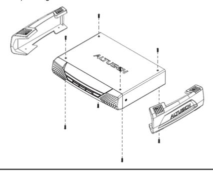
2. Remove the bottom and side screws from the KE Series transmitter unit.
