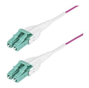
This OM4 LC to LC Multimode Duplex Fiber Optic Patch cable delivers reliable connectivity across 40 and 100 Gigabit networks. The TIA-standard Erika Violet jacket clearly distinguishes OM4 from Aqua OM3/OM4 cabling, eliminating guesswork in critical network setups. The compact uniboot connector design enables easy insertion and removal in high-density installations.
