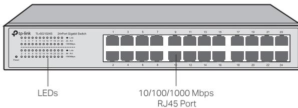
The front panel of TL-SG1024DE is shown as the following figure.
