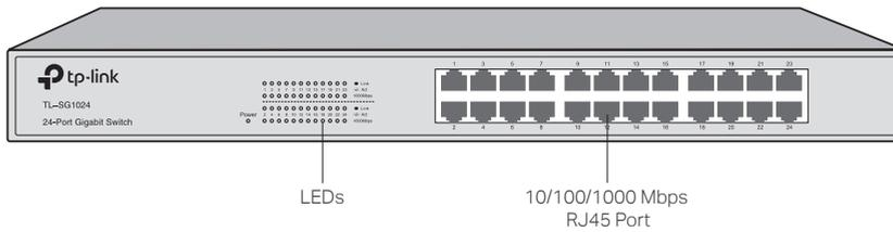
The front panel of TL-SG1024D is shown as the following figure.
