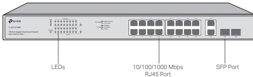
The front panel of TL-SG1218MPE is shown as the following figure.
