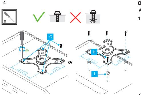
*Note:* For monitors with recessed VESA holes, the provided spacers can be used if needed.
