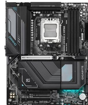
**GIGABYTE B850 GAMING X WIFI6E Motherboard - AMD Ryzen 9000 Series CPUs, 12+2+2 Phases Digital VRM, up to 5200MHz DDR5 (OC), 1xPCIe 5.0 + 2xPCIe 4.0 M.2, 2.5LAN, WIFI 6E, USB 3.2 Gen 2x2:**
