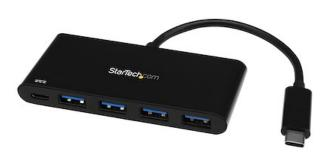
This compact USB 3.2 Gen 1 hub lets you add four USB-A ports to your laptop, with support for USB power delivery. This means that you can power and charge your laptop through its USB-C port while simultaneously powering the hub.
