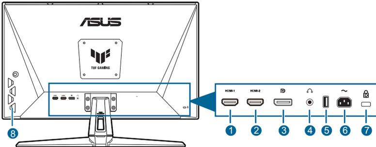
1. **HDMI-1 port.** This port is for connection with an HDMI compatible device.
