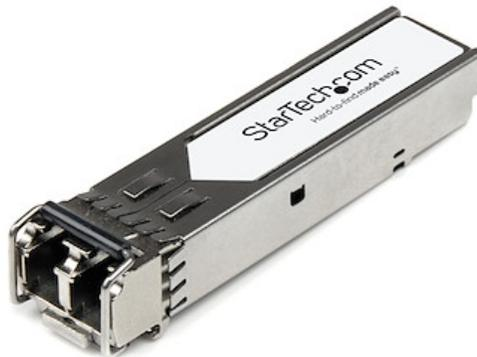
The LX-ST is a Palo Alto Networks PAN-SFP-LX compatible fiber transceiver module that has been designed, programmed and tested to work with Palo Alto Networks brand switches and routers. It delivers dependable 1 GbE connectivity over fiber cable, for 1000BASE-LX compliant networks, with a maximum distance of up to 10 km (6.2 mi).
