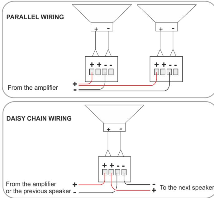
Figure 5: Open-back Ceiling Speaker Schematic Pinout Diagram
