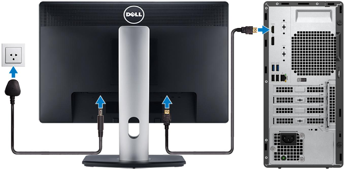
**i** **NOTE:** If you ordered your computer with a discrete graphics card, the HDMI and the display ports on the back panel of your computer are covered. Connect the display to the port on the discrete graphics card.
