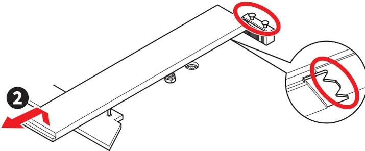
3. If you want to install the 2260 SSD, replace the **EZ M.2 Clip II** to the 2260 hole. Please note that you have to use the **EZ M.2 Chip II Remover** to remove and install the **EZ M.2 Clip II**. Skip this step if you install 2280 SSD.
