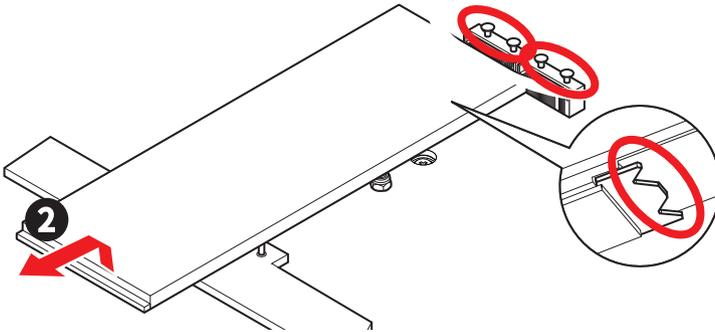
3. If you want to install the 2260 SSD, replace the **EZ M.2 Clip II** to the 2260 hole. Please note that you have to use the **EZ M.2 Chip II Remover** to remove and install the **EZ M.2 Clip II**. Skip this step if you install 2280 SSD.
