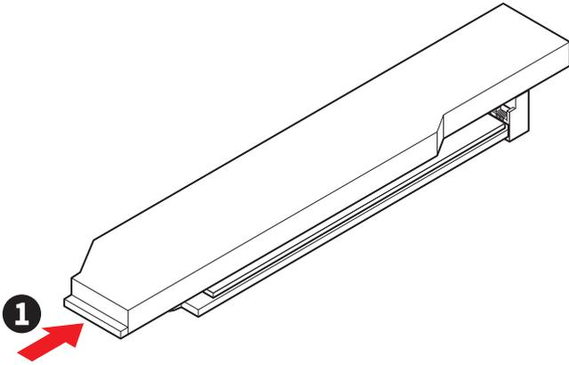
2. Slightly lift up the end part of Screwless M.2 Shield Frozr heatsink and move it forward to uninstall the heatsink.
