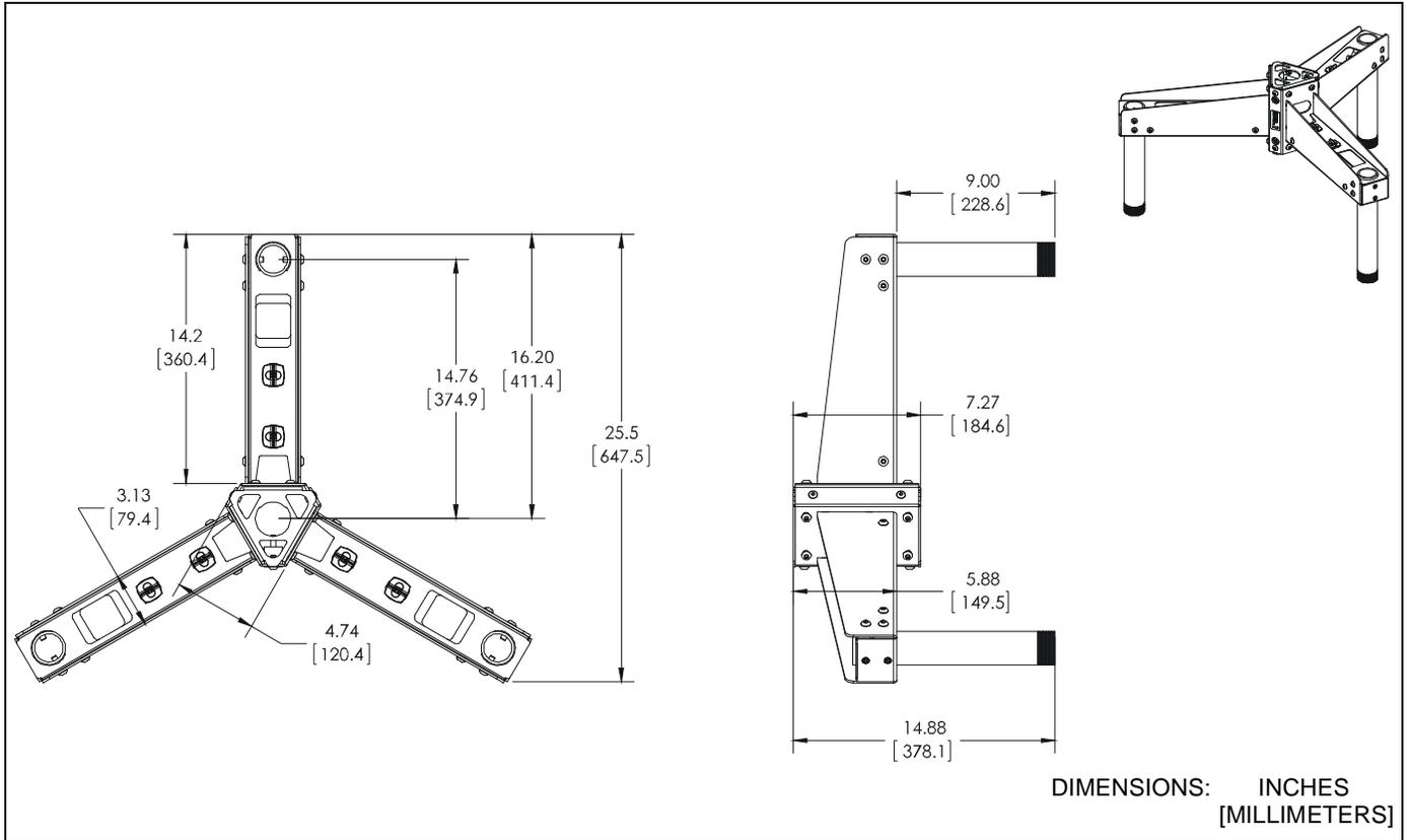
**LCM3U - Consists of FCA3U plus three LCM1U mounts**
