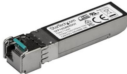
The SFP10GBBXDST is an MSA compliant downstream fiber SFP transceiver which pairs with StarTech.com's SFP10GBBXUST. They are designed, programmed and tested to work with 10GBASE-BX compatible MSA switches and routers. The SFP+ transceiver module supports a maximum distance of up to 10 km (6.2 mi) and delivers dependable 10 GbE connectivity over fiber cabling. **Technical Specifications:**
