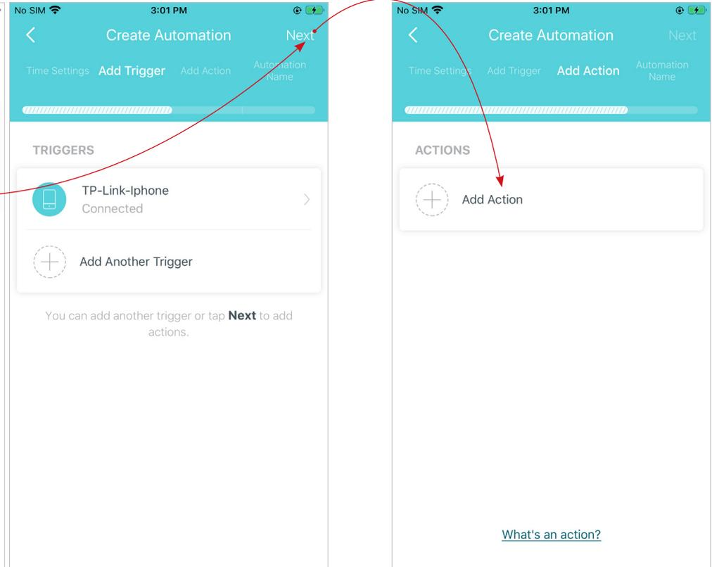
7. Select the action device and set the action details. For example, set the action as below then the living room plug will turn on after you tap the shortcut icon, and will turn off automatically after 1.5 hours.
