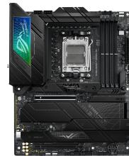
Ryzen 7000, ATX, DDR5 memory, 4x M.2, USB 3.2 Gen 2x2, PCIe 5.0, Q-Release, M.2 backplate, WiFi 6E, Aura Sync
