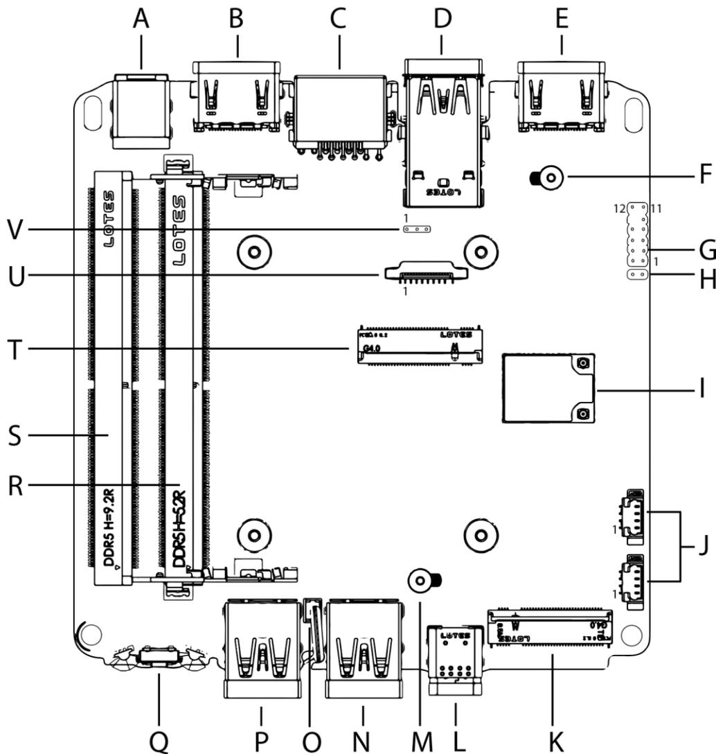
Figure 1. Major Board Components (Bottom) with Pin 1 Indicators
