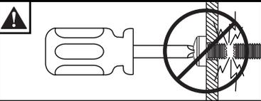
ENG Do not overtighten screws.
