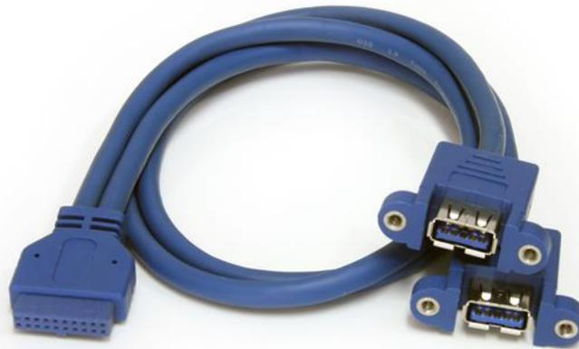
The USB3SPNLAFHD 2-Port USB 3.0 to Panel mount USB cable features a 20-pin USB 3.0 motherboard header connection on one end, breaking off into two separate USB 3.0-A (female) ports on the other end of the cable.
