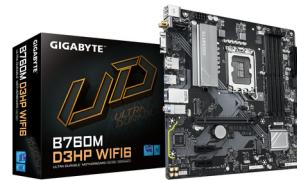
**Product name :** B760M D3HP WIFI6 Motherboard - Supports Intel Core 14th Gen CPUs, 4+1+1 Phases Digital VRM, up to 5600MHz DDR5, 2xPCIe 4.0 M.2, Wi-Fi 6, GbE LAN, USB 3.2 Gen1
