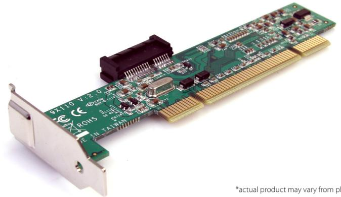
2. Install the adapter card into a PCI slot on the motherboard and secure the bracket to the computer case.
