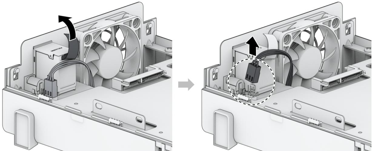
5. Remove the malfunctioning fan.
