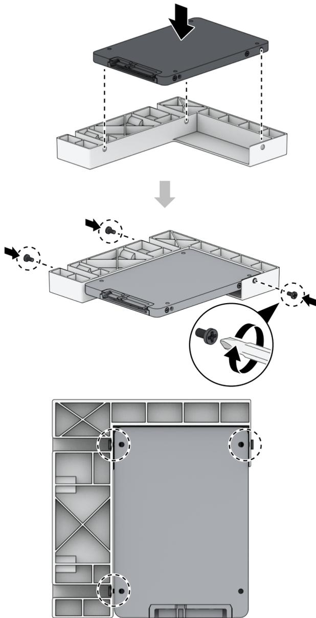
b. Slide the 2.5" Disk Holder into the hard drive bay, and push it all the way until the drive is firmly connected to the SATA connector. Secure the Disk Holder with the screws
