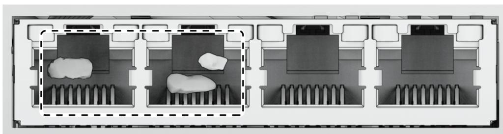
6. Check the interior of the network port for damaged or skewed pins.
