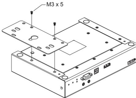
3. Screw the mounting bracket to any convenient location on the rack.
