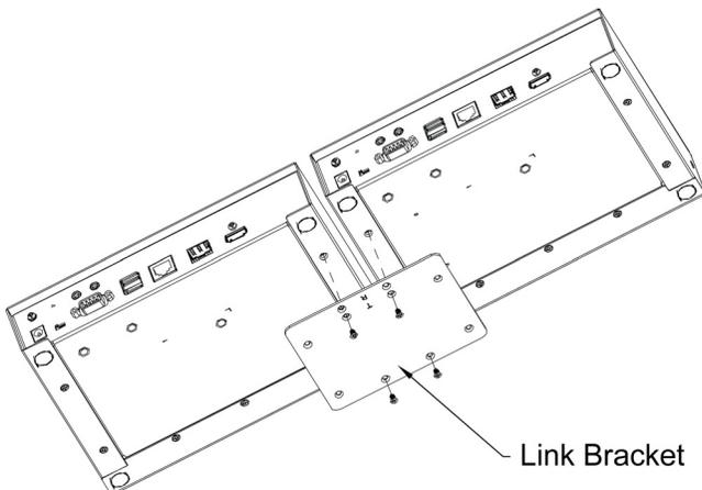
2. Remove the bottom and side screws from each unit.
