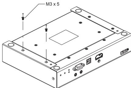
2. Use the screws from step 1 to screw the mounting bracket to the bottom of the unit.
