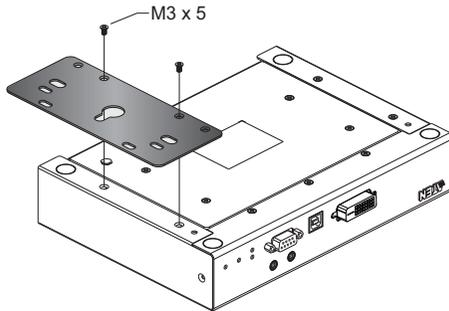
3. Use the center hole to screw the bracket to a secure wall surface.
