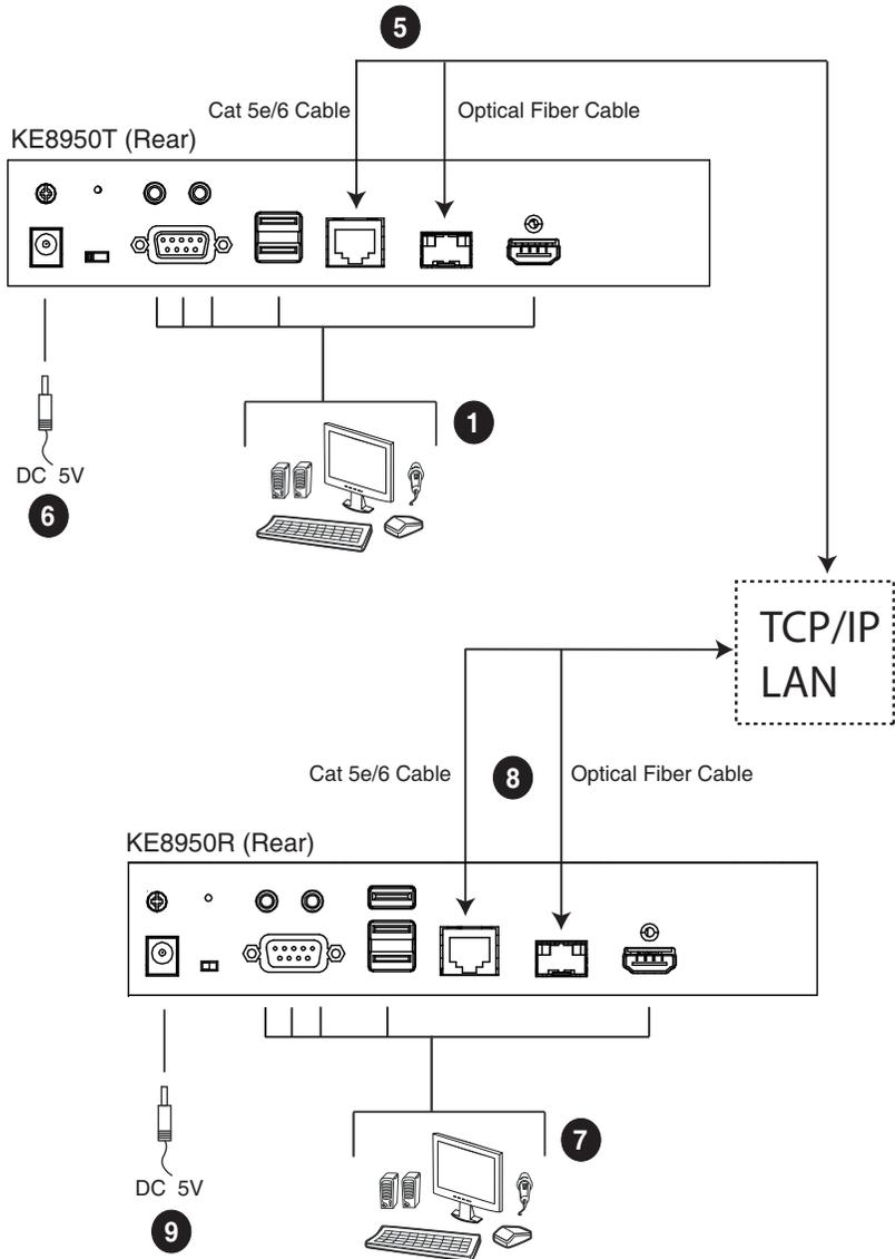
**Note:** Power adapters are not provided with KE8952 units. Please contact your ATEN dealer to purchase additional power adapters, or use the Power over Ethernet (PoE) feature to supply power to KE8952 units.
