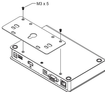
3. Use the mounting bracket's center screw hole to mount the unit on a wall.
