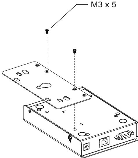
2. Screw the bracket into a convenient location on the rack.
