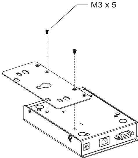
2. Use the center hole to screw the bracket to a secure wall surface.
