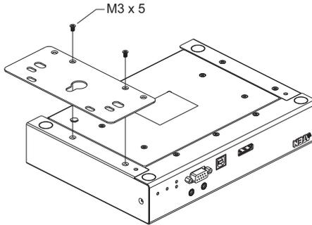
3. Use the mounting bracket's center screw hole to mount the unit on a wall.
