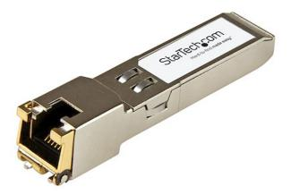
The BRSFP-1GECOPR-ST is a Brocade BRSFP-1GECOPR compatible copper transceiver module that has been designed, programmed and tested to work with Brocade brand switches and routers. It delivers dependable 1 GbE connectivity over copper cable, for 1000BASE-T compliant networks, with a maximum distance of up to 100 m (328 ft).
